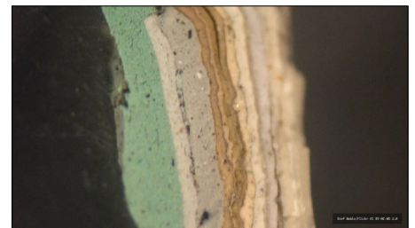
photo by: Stef Noble/Flickr CC BY-NC-ND 2.0 This microscopic image shows many generations of paint on one surface.
